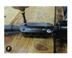
Join the 2 rope clamp sides with the longer alignment screws. If the holes are not exactly aligned, the connector body can be moved from side to side to allow the screws to be inserted. [F]
