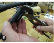
Position one half of the rope clamp between the marks. It must be configured to meet the other half and allowing the alignment of the screw holes. While avoiding damage to the clamp, push or squeeze the rope into the clamp. This may be done with a pair of pump pliers. [E]
