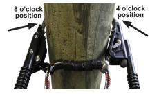
Continue step 1 until the spikes are at the 8-4 o'clock position on the pole and the nylon rollers are touching the pole.
