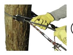
Adjust the black outer rope by holding the end of the line, grabbing the nylon handle and sliding the adjustor down the line.
