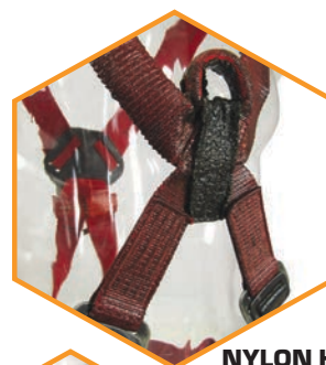
NYLON HARNESS EXPOSED TO ARC FLASH
