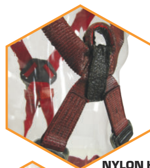
NYLON HARNESS EXPOSED TO ARC FLASH
